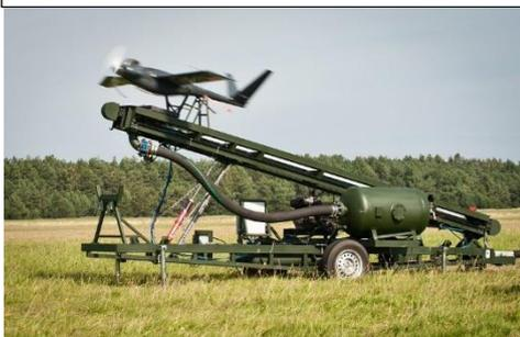
Shown on the left is an air powered launch device used for mini-UAVs like those that inspired our first concept. This device could be mounted to a truck for use in monitoring a convoy, or on the ground for monitoring a fixed location. Some mini-UAVs can be hand launched but in order to save power we felt this would be more effective. It also minimises the human intervention needed, since larger drones currently require three or more personnel to control from the ground.
